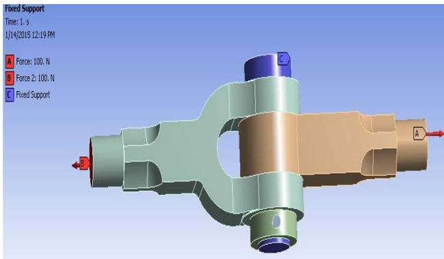
Fig. 6: Constraining conditions of knuckle joint
