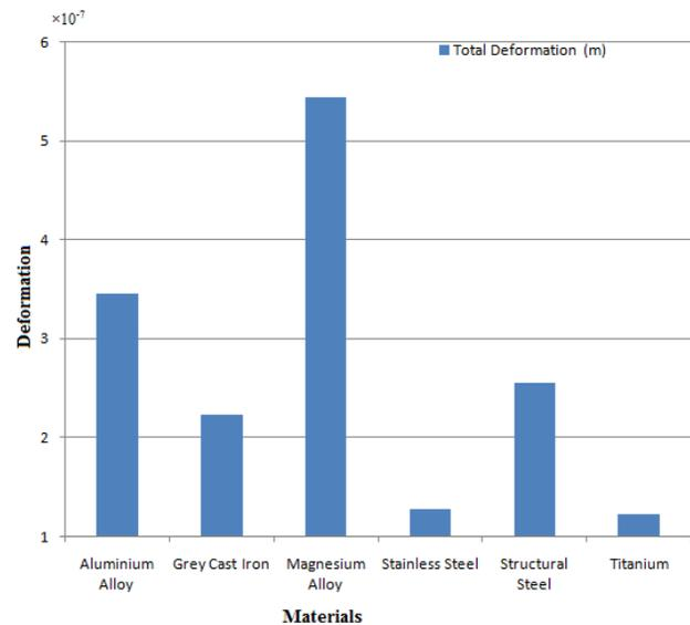
Fig. 10: Variation of deflection for different materials of knuckle joint
