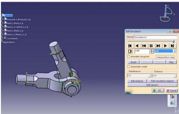
Fig. 4: Simulation of the knuckle joint using DMU kinematics
