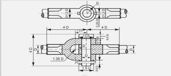
Fig. 2: Schematic of knuckle joint
