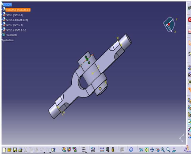
Fig. 3: 3-d CAD modelling and Assembly of the knuckle joint
