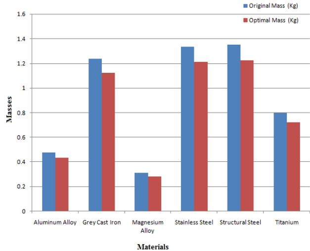
**Fig. 13: Variation of different masses for different materials of knuckle joint**
