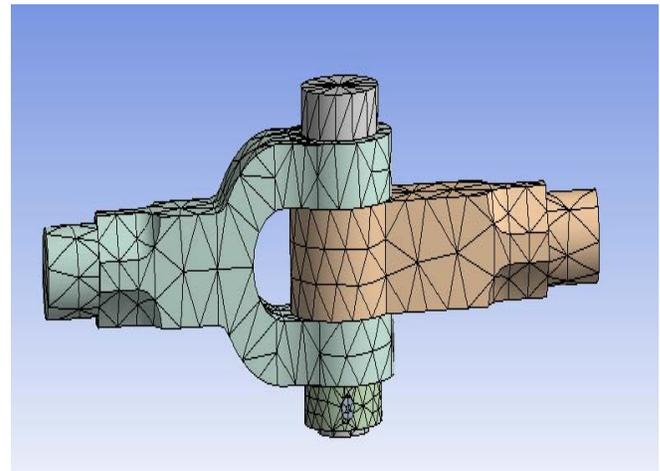
Fig. 5: Meshing of knuckle joint
